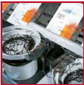
Double automatic hanger feeder
